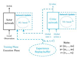
Figure 2: Actor and critic networks of one agent during training and execution phases.
