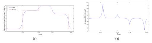
Figure 4: (a) Average charge and discharge and (b) average state of the charge (SOC) of batteries in the whole fleet for one day in a representative region and time period after LQG calibration.
